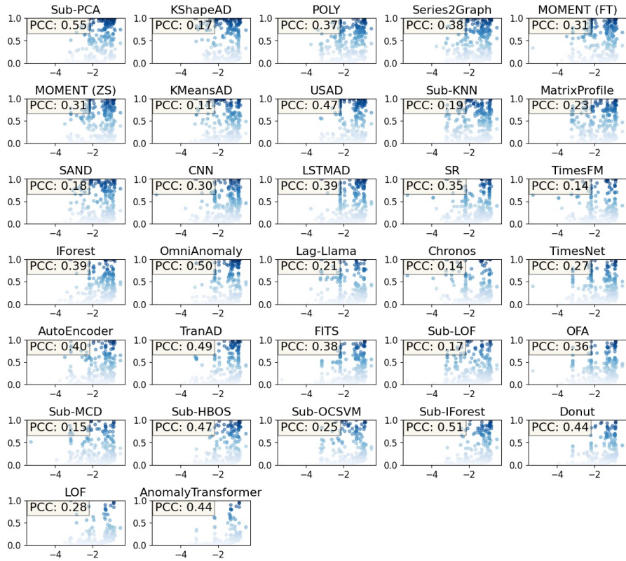
Figure 13: Influence of anomaly ratio on model performance in TSB-AD-U. PCC indicates the Pearson Correlation Coefficient.
