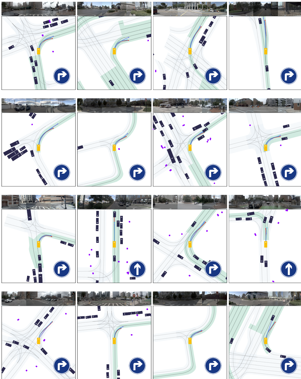
Figure 7: NAVSIM Results: DP-VLA w/ DIPOLE fine-tuned model trajectory; ground truth ego trajectory; DP-VLA imitation pretrained model trajectory.
