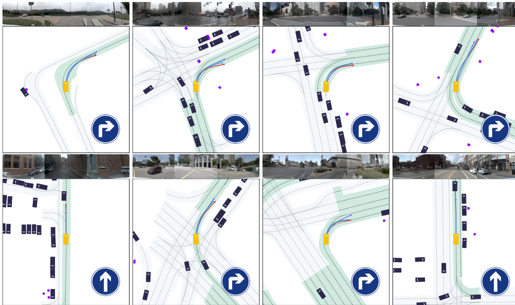
Figure 2: NAVSIM Results: DP-VLA w/ DIPOLE fine-tuned model trajectory; ground truth ego trajectory; DP-VLA imitation pretrained model trajectory.
