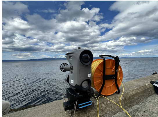
Fig. 2. Data collection platform. The Blueeye X3 ROV with a tether reel. The ROV carries a monocular camera, an Oculus M750d multibeam sonar, and onboard temperature and pressure sensor.
