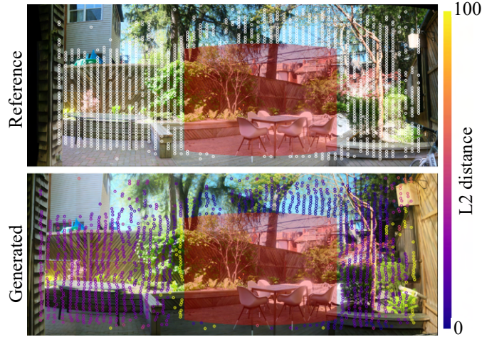
Figure S3: Example of LoFTR feature matching between reference and generated panoramas. White circles mark selected keypoints in the reference, with corresponding points in the generated panorama color-coded by L2 pixel distance from their reference positions.
