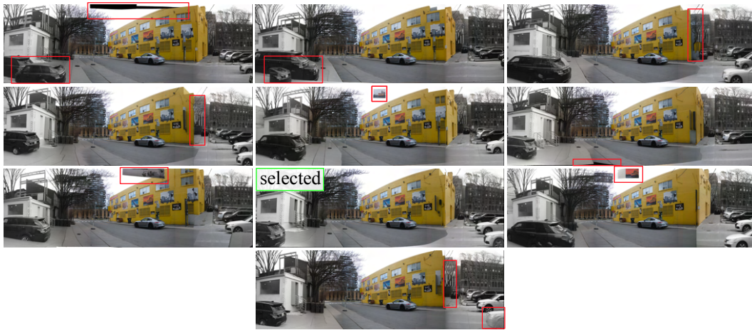
Figure S5: Example of the correspondence-based seed selection strategy to generate the full panoramic canvas. We generate 10 panoramas with different seeds and select the one with most feature matches. The selected panorama has the least artifacts in this example and is the most seamless and similar to the reference.
