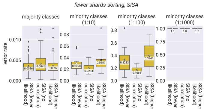
Fig. 8. Results for adaptive assignment into fewer shards. Higher/lower likelihood refers to the likelihood of the minority classes. All models have 5 shards and 3 slices.
