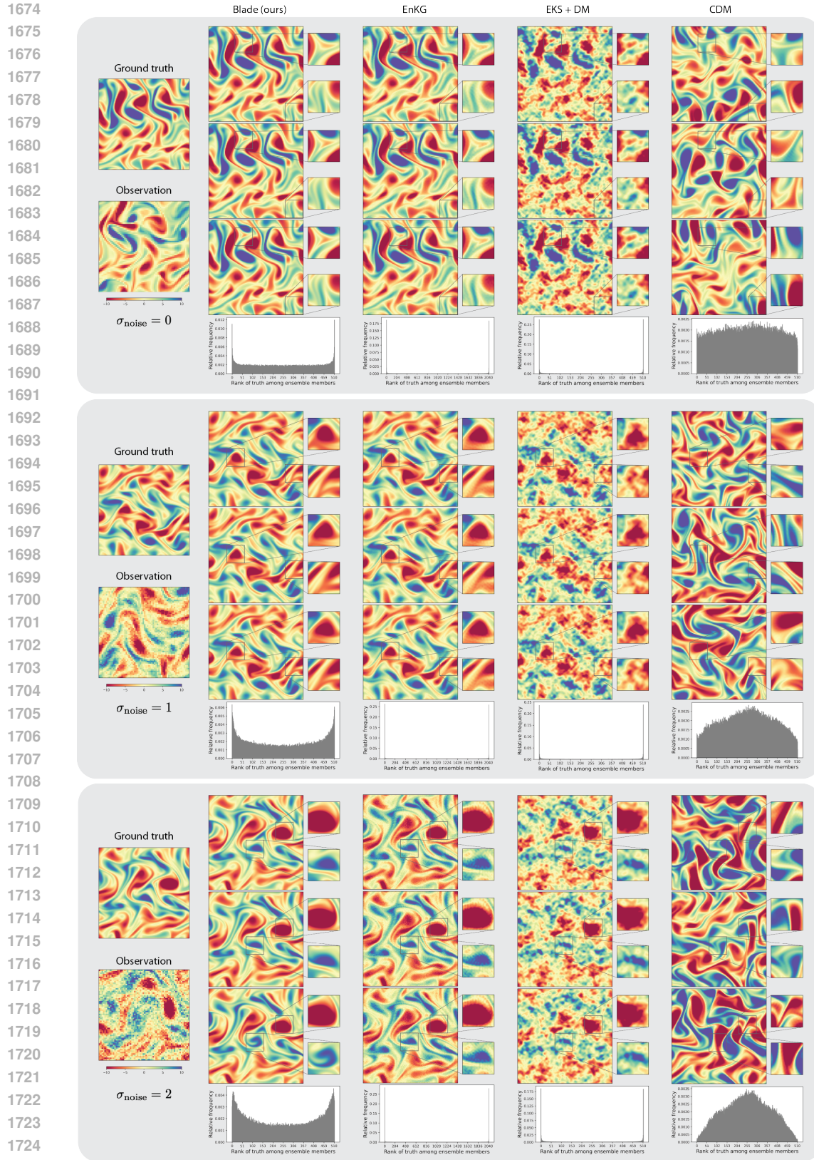
1726 Figure 9: Qualitative and probabilistic assessment on Navier-Stokes inverse problem at three observation 1727 noise levels. Each block presents qualitative results with zoom-in views and the rank histogram calculated over all test cases. Blade produces the flow structures accurately while capturing realistic local variability, and its rank histogram demonstrates superior ensemble calibration.
