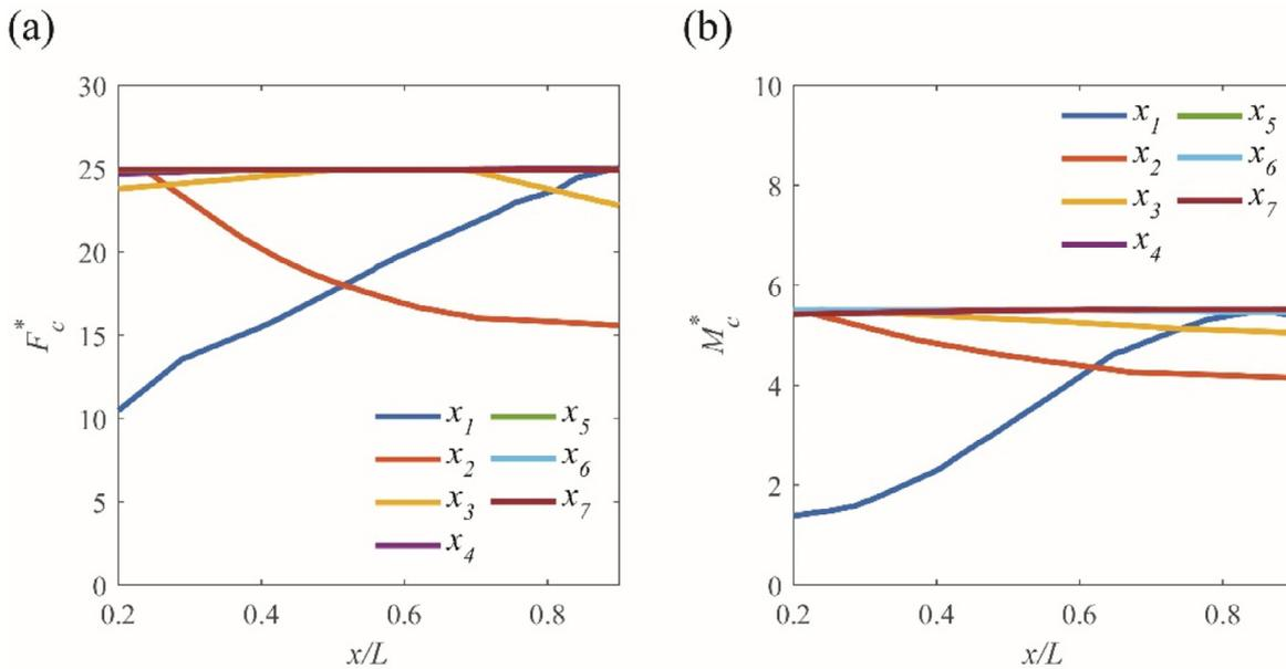
**Fig. 4.** (a) The critical normal force  $F_c^*$  as a function of each control point position. Each curve corresponds to varying the position of one control point with other control points kept the same as the design in Fig. 2(a). The critical moment  $M_c^*$  as a function of each control point position. Each curve corresponds to varying the position of one control point with other control points kept the same as the design in Fig. 3(a).
