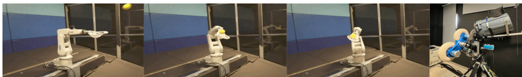
Figure 1: Mobile Manipulator with Lacrosse Head catching a ball within a second. (right) Automatic ball thrower with controllable yaw angles and speed of around 5m/s.
