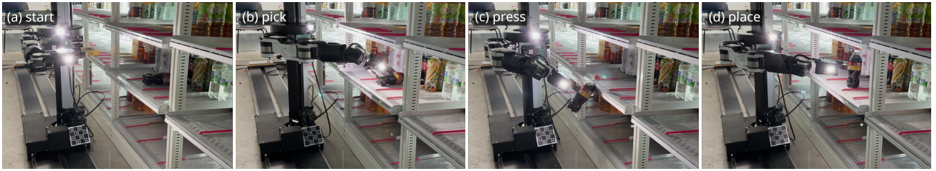
Fig. 3. Bottle-recovery task decomposed into four stages: (a) Start —initial state, (b) Pick —approach and grasp the bottle, (c) Press —move to the shelf edge and press the bottle against it, (d) Place —move to the shelf and set the bottle upright.
