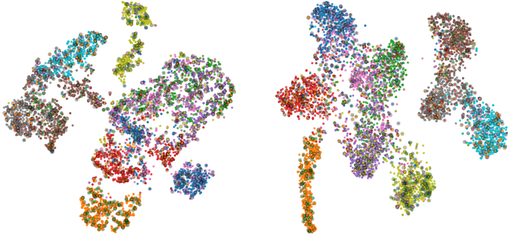
(a) Embeddings from the raw feature space show overlapping class clusters, with noisy samples (circled) indistinguishable from clean ones. (b) Embeddings after Siamese training: clean samples form compact, well-separated clusters, while noisy samples shift to the periphery or inter-class regions.
