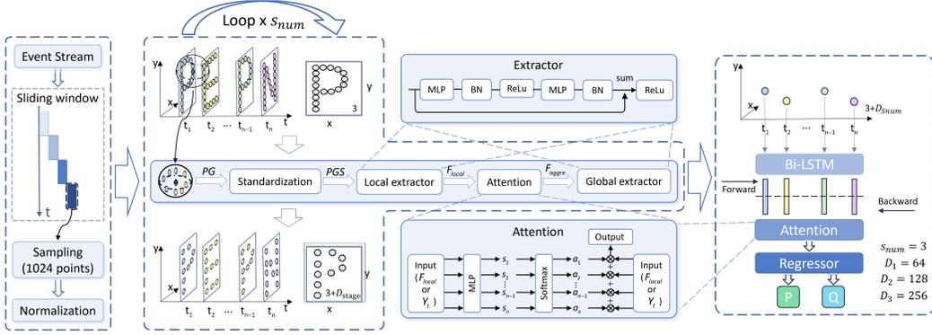
Figure 3: PEPNet overall architecture. The input Event Cloud undergoes direct handling through a sliding window, sampling, and normalization, eliminating the need for any format conversion. Sequentially, the input passes through  $S_{num}$  hierarchy structures for spatial feature abstraction and extraction. It further traverses a bidirectional LSTM for temporal feature extraction, culminating in a regressor responsible for 6-DOFs camera pose relocation.
