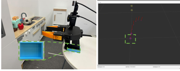
Figure 10: Left: The blue 3D-printed groove on the table, serving as a clear visual reference to aid loop closure. Right: The T265’s trajectory in RVIZ, illustrating alignment with the initial reference, highlighted as a green dashed box, after revisiting the blue groove.
