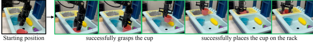
Figure 8: Evolution of learned behaviors during online fine-tuning of diffusion policies with PA-RL on task (a). The offline BC policy (in red) fails to even grasp the cup. During intermediate online interaction episodes (in yellow), it successfully grasps the cup, but fails to place it on the rack. After 50 episodes (in green), it learns to successfully grasp the cup and place it on the rack.
