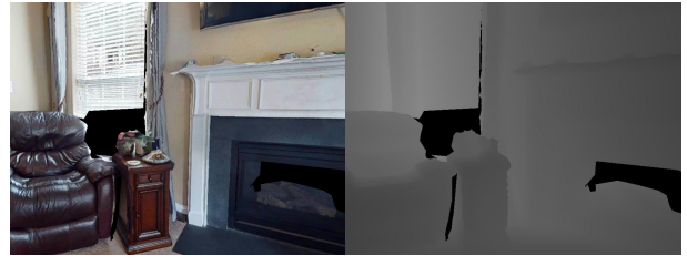
Fig. 6. An example of reconstruction artifacts (or defects) found in real-world scan datasets. The depth image (right) shows significant data loss so called ‘holes’ or ‘black cracks’.
