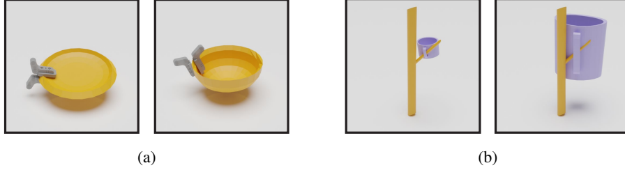
Figure 5: Predicting grasps using interaction point warping. (a) the predicted grasp for a bowl/plate changes based on the curvature of the object. (b) the placement of a mug on a mug tree changes as the mug grows larger so that the branch of the tree is in the middle of the handle.
