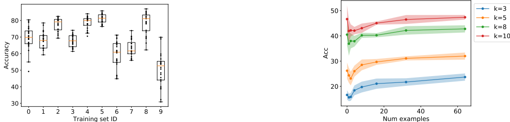
Figure 7: (Left) In-context accuracy varies widely with example ordering. Each training ID refers to a set of training examples. Each dot refers to the in-context learning accuracy of one permutation of the training examples for that particular training ID. (Right) Zero-shot performance can be higher than one/few-shot performance in some settings in GINC, mirroring the behavior of GPT-3 on some datasets such as LAMBADA (Brown et al., 2020). The few-shot setting introduces the distracting prompt structure, which can initially lower accuracy.
