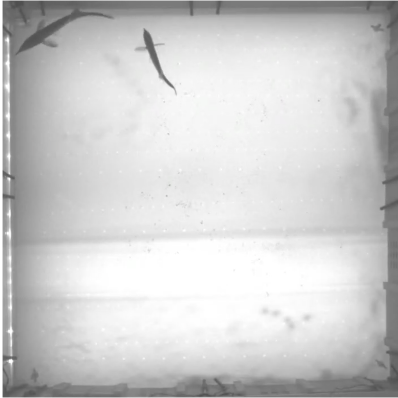
Figure 4: A screenshot from the tank from which our data was collected. The dark vertical slabs along the wall are the electrode sensors.
