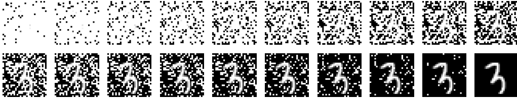
Figure 13: Nosaic MNIST (NMNIST) database consists of videos of 20 frames, each of which has 28 \times 28 \times 1 pixels. The frames are buried with noise at the first frame, gradually denoised toward the last frame. NMNIST provides a typical task in early classification of time series.
