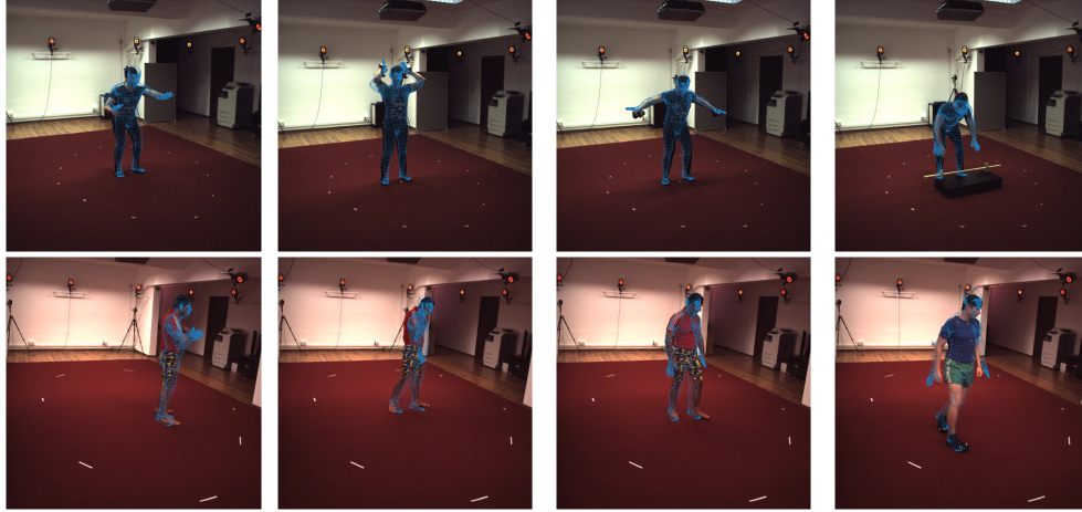
Figure 7: Qualitative results when projecting the SMPL body model from the OSDCap poses back to the input 2D images. The overlaid SMPL models are shown in sparse blue point cloud to maximize the visibility of the input human pose.
