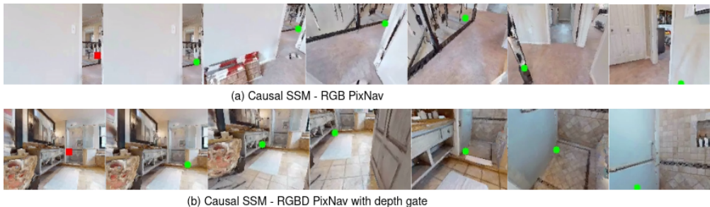
Figure 6: Goal pixel tracking capability of (a) Causal SSM-RGB PixNav, (b) Causal SSM-RGBD PixNav with depth gate is shown for random pixel goals in HM3D scenes. Pixel goal (red) and predicted goal coordinate (green) during rollout validation for episode images at different timesteps. It is clear that the Causal SSM-RGB PixNav model tracks the goal pixel more consistently. As depth gate regulates geometric cues, tracking relies primarily on appearance-based feature continuity. Additionally, temporal feature modulation introduced by depth gating might have slightly affected the stability of the representations passed to the Mamba layer.
