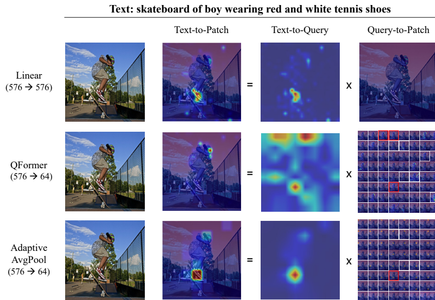
1072 (b) R-GAE maps related to the generated text “skateboard of boy wearing red and white tennis shoes” are shown 1073 in Figure 10. In this case, the QFormer-based MLLM fails to attend to the relevant patches with the “red and 1074 white tennis shoes” attributes. In contrast, both the linear projector and the AdaptiveAvgPool highlight the 1075 correct patches.
