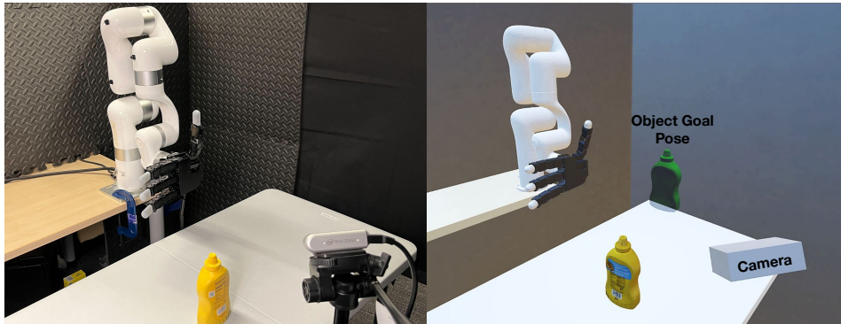
Figure 2: Our Dexterous Manipulation System. Left: Real-world setup with an Allegro Hand attached on an XArm6 and a RealSense D435. Right: Simulator setup with the transparent green object representing goal pose.
