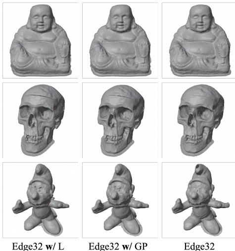
Figure 6: Comparisons of our three fitting methods, linear interpolation (L), Gaussian Process (GP), and no interpolation. The linear interpolation method produces the best results numerically and visually.
