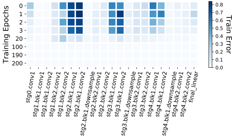
Figure 2: Analysis of rewinding modules to initialization for the ResNet-18 architecture. Each row represents a module in ResNet18-v1 and each column represents a particular training epoch to which this module is rewound to. The difference from analysis of Zhang et al. (2019a) is that we rewind each module, whereas Zhang et al. (2019a) rewind the entire ResNet blocks.
