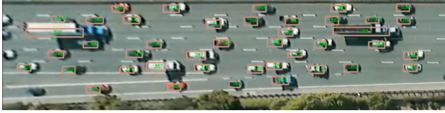
Figure 3. A snapshot of vehicles tracked in NGSIM. The bounding boxes denote the positions of tracked vehicles (their numbers are NGSIM indices).
