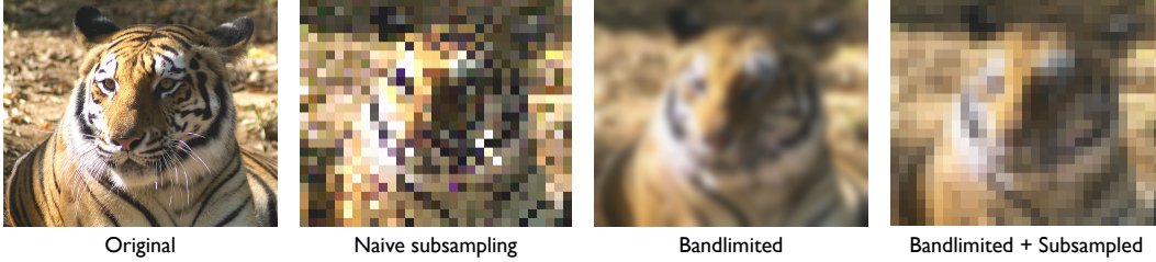
Figure 1: How to correctly downsample an image. Left to right: The original high-resolution image; an \times 1/8 subsampled image, notice how a lot of the image structure has been destroyed; a high-resolution, bandlimited (blurred) image; a bandlimited and \times 1/8 subsampled image. Compare the bandlimited and subsampled image with the naïvely subsampled image. Much of the low-frequency image structure is preserved in the bandlimited and subsampled image. Image source: ImageNet.
