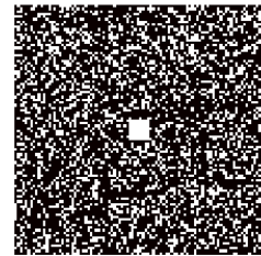
Figure 1: Undersampling mask used in this study (white signifies measured Fourier coefficients, black signifies skipped coefficients).
