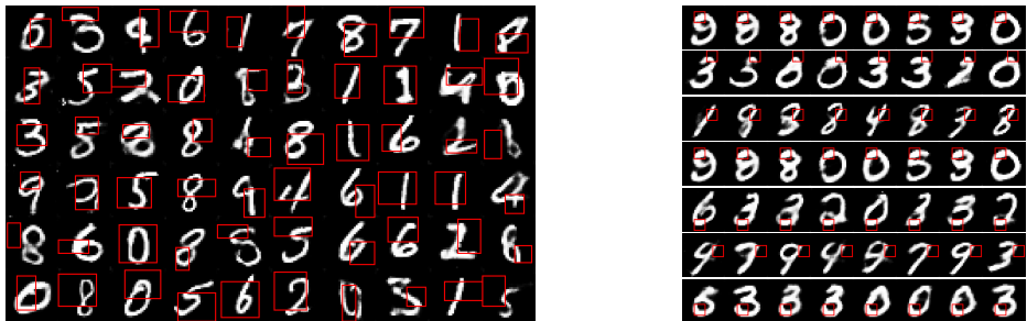
Figure 8: Inside of each red box are the observed pixels; the pixels outside of the box are generated by the imputer. Right: each row corresponds to the same incomplete input, marked by the red box.
