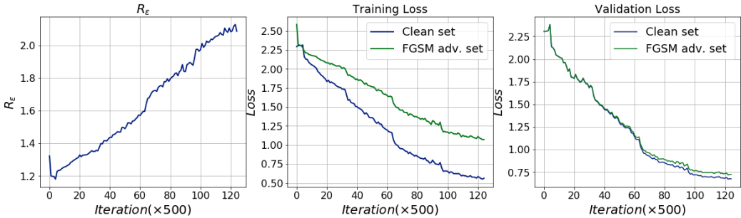
Figure 11: CIFAR-10 : Trend of R_\epsilon , training loss, and validation loss during SADS training method, obtained for ResNet-34 trained on CIFAR-10 dataset using SADS. Column-1: plot of R_\epsilon versus training iteration. Column-2: training loss versus training iteration. Column-3: validation loss versus training iteration. Note that, for the entire training duration R_\epsilon does not decay, and no over-fitting effect can be observed.
