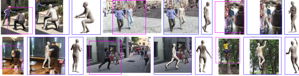
Figure 5: Qualitative results. The input is shown with a magenta detection box identifying the person at its center. Blue boxes show the output of our Motion HMR model. We show both the image-aligned estimated mesh, and the same mesh rotated by 60 degrees. Note that our algorithm is robust to both unusual poses (top left; bottom right) and occlusions (top right; bottom left).
