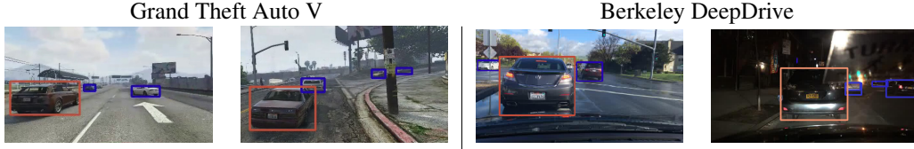
Figure 1: Our method uses discrete objects as part of the policy model for driving in traffic. The learned selector identifies the objects most relevant to the policy, which is often the nearest car.
