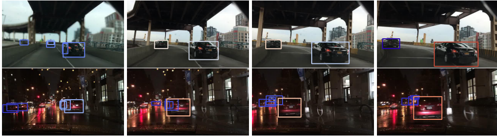
Figure 6: Sample scenes from the Berkeley DeepDrive Video dataset with the sparse model’s learned selector visualized. Red indicates a high scoring object, and blue is low scoring (best viewed on screen). Our method is robust to imperfect detections, such as overlapping bounding boxes, for both day and night scenes.
