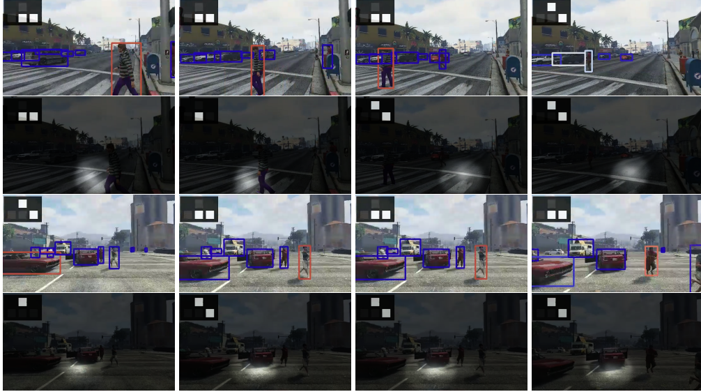
Figure 5: Sample scenes from the Grand Theft Auto V simulation with our sparse model’s learned object selector compared against a learned pixel-level attention. For rows 1 and 3, red indicates a high scoring object, and blue is low scoring (best viewed on screen). For rows 2 and 4, then pixel attention is shown by brightness of the pixels. The actions output by each model are shown by the white squares in the corners: accelerator is the top square, and the bottom squares are turn left, brake, and turn right, respectively. A single action may both turn and accelerate or brake. Rows 1 and 2 shows both models performing well, while rows 3 and 4 show the pixel attention model ignoring pedestrians and deciding to accelerate towards them. The object centric model is more conservative and attends strongly to the pedestrians, choosing to slow down instead of speeding up.
