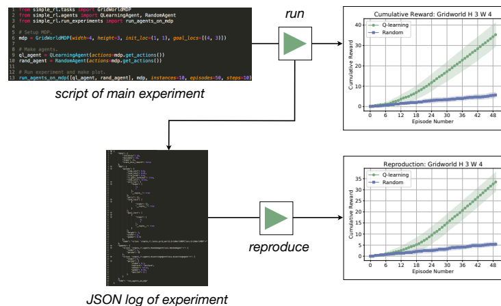
Figure 1: The core functionality of simple_rl : Create agents and an MDP, then run and plot their resulting interactions. Running an experiment also creates an experiment log (stored as a JSON file), which can be used to rerun the exact same experiment, thereby facilitating simple reproduction of results. All practitioners need to do, in theory, is share a copy of the experiment file to someone with the library to ensure result reproduction.
