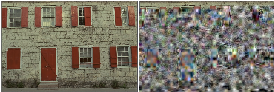
Figure 1: The same image, decoded with a model computing the prior using integer arithmetic (left), and the same model using floating point arithmetic (right). The image was decoded correctly, beginning in the top-left corner, until floating point round-off error caused a small discrepancy between the sender’s and the receiver’s copy of the prior, at which point the error propagated catastrophically.
