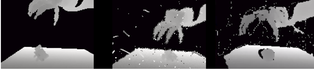
Figure 13: Left: clean depth image from the simulator. Middle: depth image from the simulator after added noise. Right: depth image in the real world (different object from the left two images).
