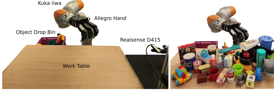
Figure 3: The robot platform consists of an Allegro hand mounted to a Kuka LBR iiwa arm, one Intel Realsense D415 camera, a work table, and a bin to drop grasped objects.
