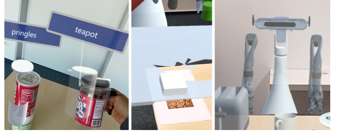
Fig. 3: Left: real object recognition via AR markers; Middle: AR marker anchoring the virtual robot in the real world; Right: the position and orientation of the virtual robot w.r.t. the teacher is used to control the reaction to teacher’s behaviour.
