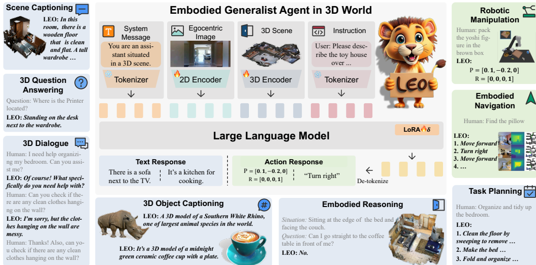
Figure 1: The proposed embodied generalist agent LEO. It takes egocentric 2D images, 3D point clouds, and texts as input and formulates comprehensive 3D tasks as autoregressive sequence predictions. By fine-tuning LEO, it extends the capability of LLMs to multi-modal vision-language-action tasks with a unified model.
