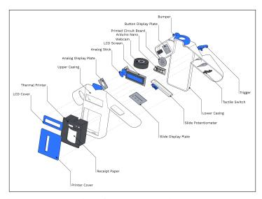
Figure 1: Exploded view of the components in Large Language Label
