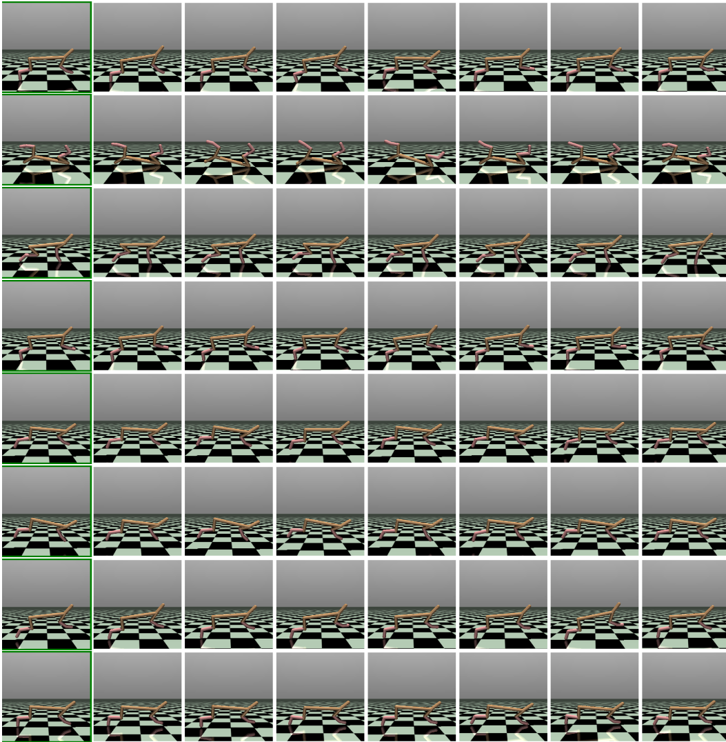
Figure 5: State similarity learned by PLOFF for HalfCheetah on the medium-replay dataset. For each row, the leftmost image is the state for which we compute nearest neighbors in the dataset \mathcal{D} for the metric induced by \Psi (ranked by decreasing level of similarity).
