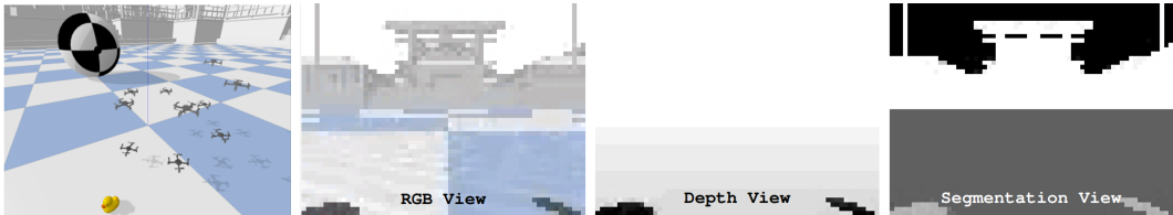
Figure 2: Overview of Multi-Agent Quadcopter Control environment and the observation for the quadrotor. A quadrotor is (i) an easy-to-understand mobile robot platform whose (ii) control can be framed as a continuous states and actions problem but, beyond 1-dimension, (iii) it adds the complexity that many candidate policies lead to unrecoverable states, violating the assumption of the existence of a stationary state distribution on the entailed Markov chain.
