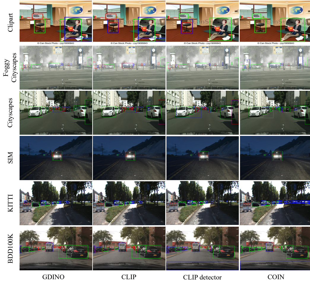
Figure 5: Qualitative results on Clipart, Foggy-Cityscapes, Cityscapes, SIM, KITTI and BDD100K. Green, red and blue boxes represent true positives (TP), false negatives (FN) and false positives (FP), respectively. Zoom in for best view.
