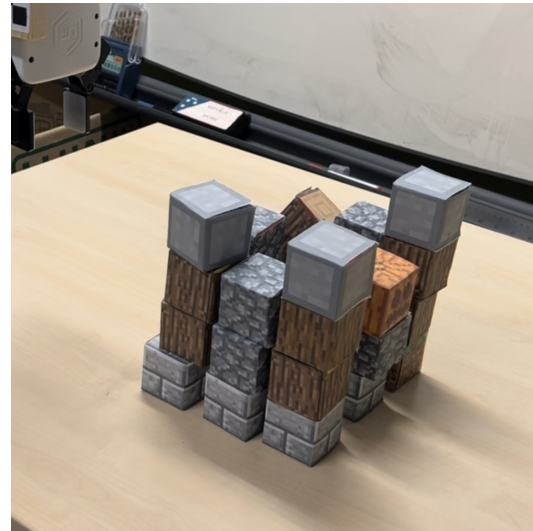
(g) A 28-block Castle. Note that the robot failed to stack two blocks properly towards the back left. In the end 26 out of 28 blocks were stacked
