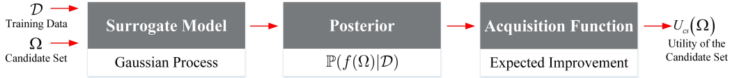
Figure 5: Pareto representation improvement scheme based on BO algorithm. The surrogate model for the objective function f(\Omega) is typically a Gaussian Process. Posteriors represent the confidence a model has about the function values at a point or set of points. Acquisition function is employed to evaluate the usefulness of optimal guess point corresponding to posterior distribution over f(\Omega) . The expected improvement method chosen to design the acquisition function in our scheme.
