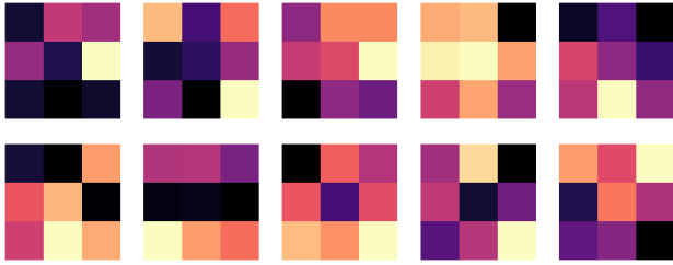
Figure 1. A subset of first-layer filters for the MNIST dataset. Single-channel weights are normalized with a z-score, clipped at \pm 3\sigma , and visualized using a 'magma' colormap.
