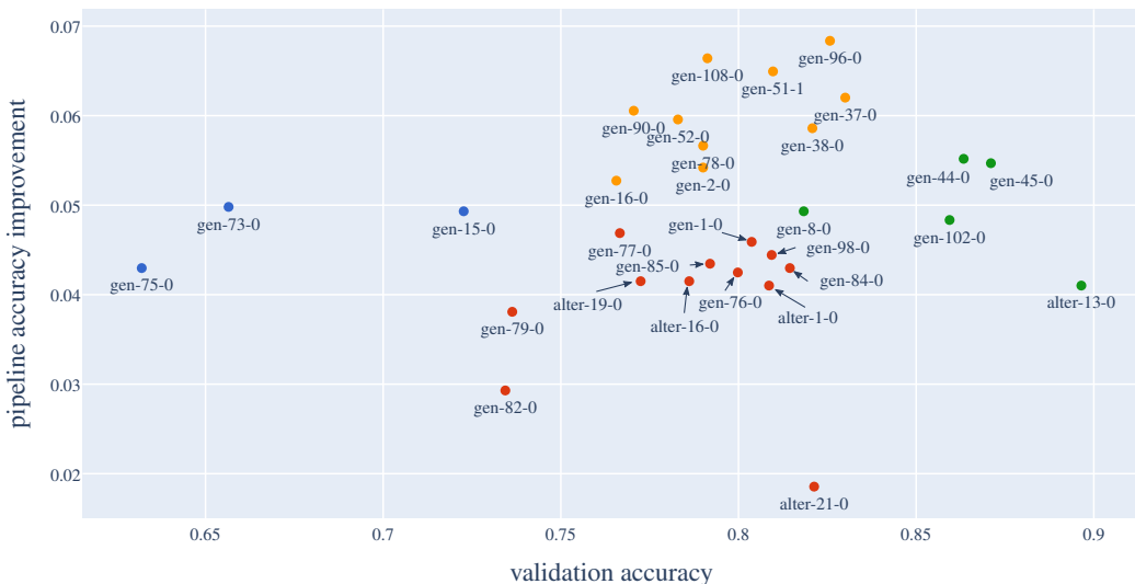
Figure 16: Pipeline accuracy improvement (percentage points) compared to validation accuracy of all trained models. Colors are based on k-means clustering with 4 clusters.
