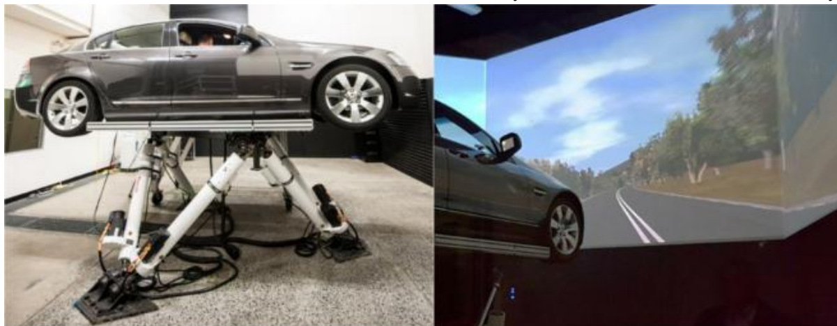
Figure 1. CARRS-Q advanced simulator used for our data collection. The simulator consists of a car with an automatic transmission, front view (180-degree), rear-view mirrors, audio system, and hydraulic system to simulate vehicle motion, and a BIOPAC system to obtain physiological signals.
