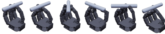
Figure 3: Visualization of canonical grasp. Inspired by how humans spin pens, we design six canonical initial poses used to reset the episode. These poses are keyframes where each finger breaks and re-establishes contact.
