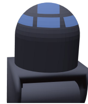
Figure 5: Touch sensor (blue) arrangement.
