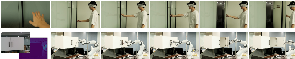
Figure 1: Our policy learns to infer object motion and intrinsic from history observation, following how humans open a door even with covered eyes. Our impedance-aware policy achieves 84% success rate in the real world, using only one first-frame RGBD image.
