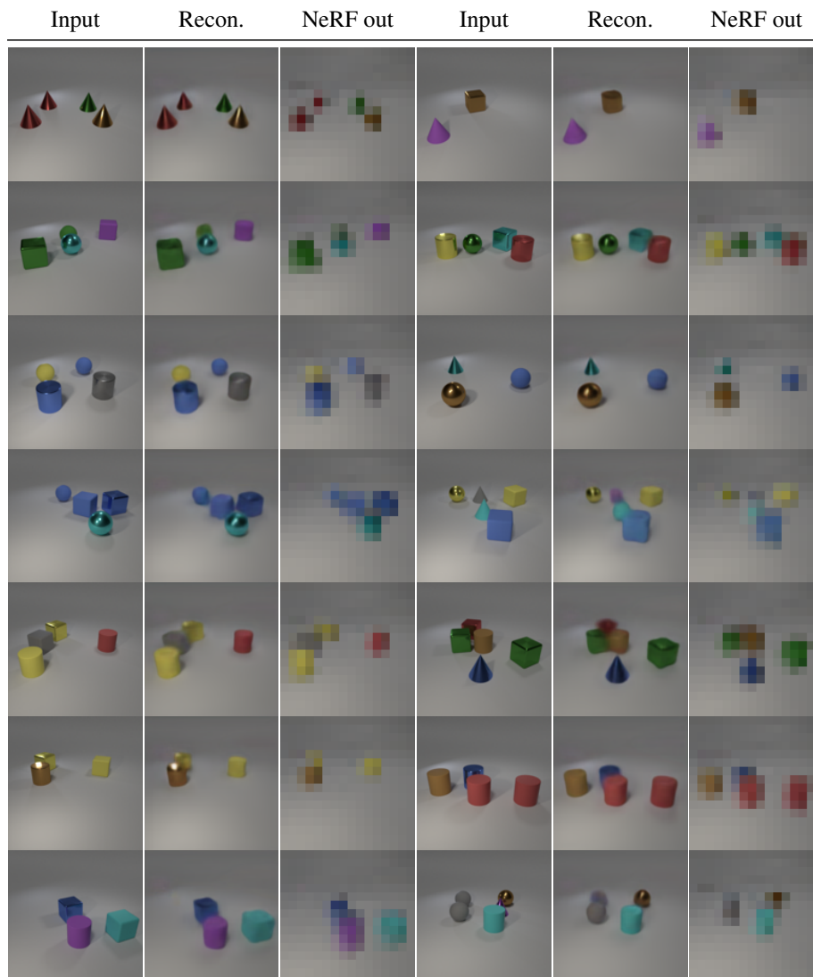
Figure 7: NeRF outputs on CLEVR2345 . For each input scene we show the reconstructed image as well as each the low resolution output of the NeRF function. This output is then upscaled with a neural network to obtain the reconstructed scene. While NeRF output lack full detail, they correctly depict each individual object and their position in the scene.
