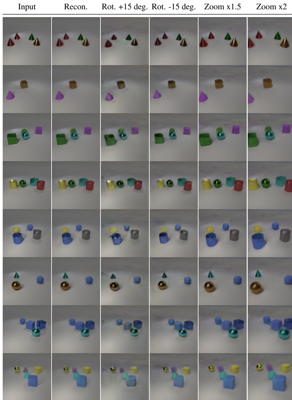
Figure 6: Novel view synthesis on CLEVR2345. For each scene, we move the camera \pm 15^\circ on the azimuth axis. Additionally, we zoom in the scene twice. While our model is trained with a fixed default camera pose and single scene views, it is able to generalize to small camera pose modifications and render novel views of a scene.
