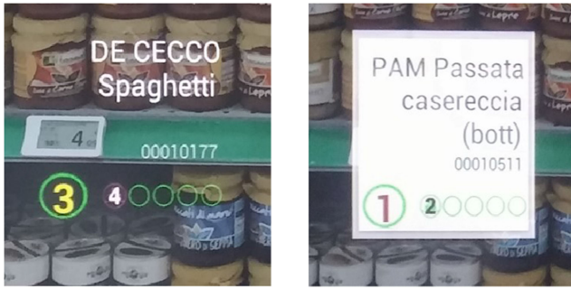
Fig. 5. View from AR headset for (left) central transparent (right) and central opaque backgrounds [19].
