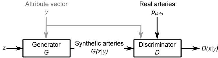
Figure 1: Overview of the proposed method for coronary artery synthesis. The generative adversarial network consists of a generator network G that transforms noise vectors z from a latent probability distribution p_z into a 4-channel 1D parametrization of a coronary artery. These representations are compared with those of real arteries in a discriminator network D , which tries to predict a high score for real arteries and a low score for synthesized arteries. In addition, the generator and discriminator can be conditioned on an attribute vector y containing information about the real or synthetic samples.
